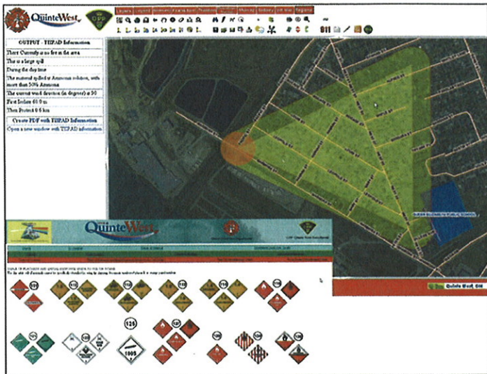
An area of isolation based on a chemical spill is delineated using the TIIPAD Tool which triggers a telephone notification to residents.
